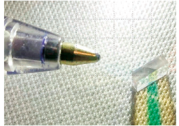
FIGURE 8: Miniaturized PBS cube for near-eye display applications.
