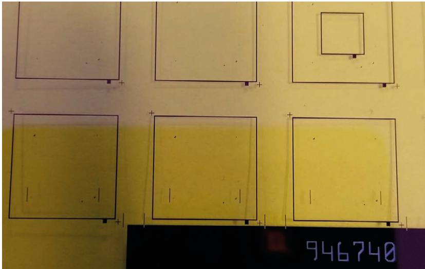
FIGURE 2: Wafer scale manufactured customized substrate with AR coating, serial numbers and chrome alignment patterns.
